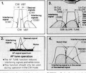
1) CW Variable Bandwidth Tuning. Vary the passband width continuously in the CW, FSK and AM modes, without affecting the center frequency. This effectively minimizes QRM from nearby SSB and CW signals
